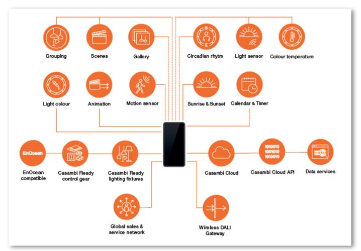
Casambi is an advanced lighting control solution based on Bluetooth Low Energy (BLE). Bluetooth Low Energy is the only low power wireless technology in all modern smartphones, tablets, and even smart watches, making it the only mainstream and future proof low power radio technology in the world.
